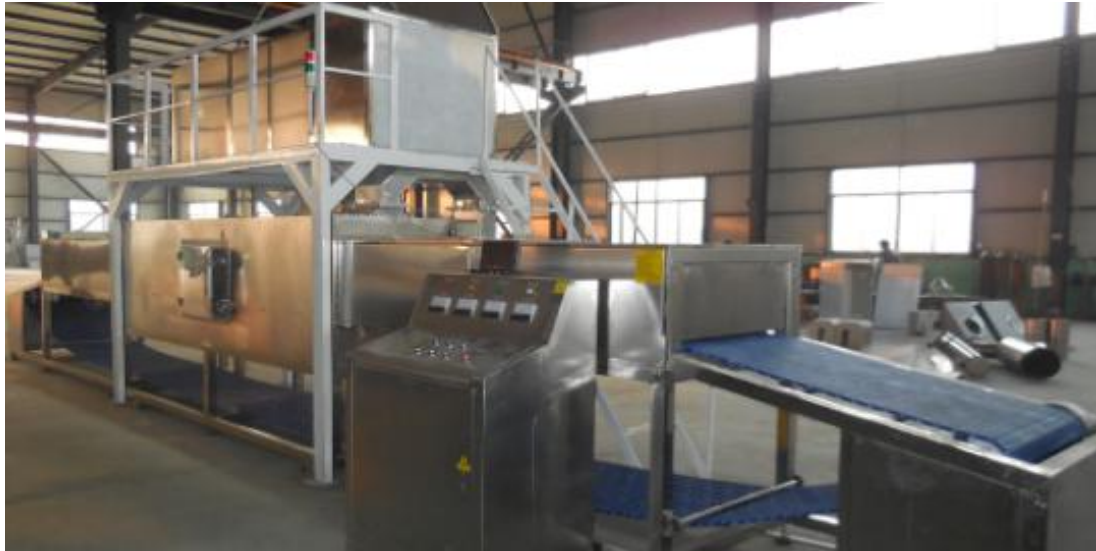
Industrialized microwave thawing equipment
